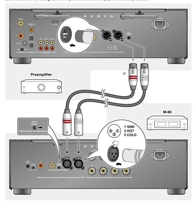
•To remove the XLR cable from this unit, press and hold the connector button (b), and pull the cable.
