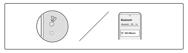
• When connecting multiple BLUETOOTH-supported devices, cancel the current connection, or press and hold the BLUETOOTH button of the remote controller for three seconds to let the unit enter the pairing standby mode. Then turn on the BLUETOOTH function of the next device.
