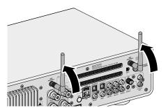
► Point the antennas upwards.
