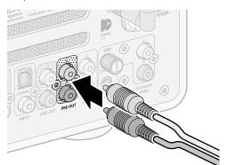
► Insert the plugs into the appropriate connection sockets.
