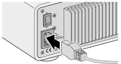
▶ Plug the power cable into the device.
