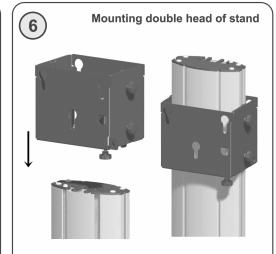
Slide the double head of the stand from the top downwards by using the T-ducts on both sides of the column. Tight the knobs on the right and left-hand side of the head to fix on a specific height.
