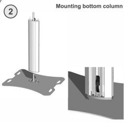
Place the bottom column of the stand (cable duct closed) carefully on the foot plate. Use the latch to secure bottom column to the foot.
