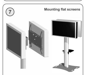
a bracket with three coupling boxes has to be mounted at the back of the flat screens (see specific mounting instructions flat screen brackets)
