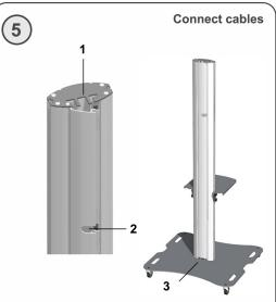
The cables can be guided through the cable duct(s). The cables can come out of the ducts at the top of the column (1) or out of the cover gab (2). The other side of the cables can come out of the bottom end of the column (3). All cable ducts have to be closed.
