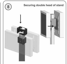
Slide the securing profile over the double head of the stand (when cables come out of the top of the column the cables must be put firstly through the securing profile). The double head of the stand and the securing profile can be locked at the side with an optional anti-theft lock.
