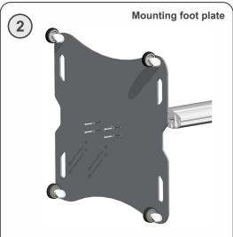
Mount with at least two persons the footplate with 4 bolts (M8x40) and 4 washers to the column. One person is holding the column and the other person is holding and mounting the foot plate. Use a threadlocking fluid to secure the bolts.
