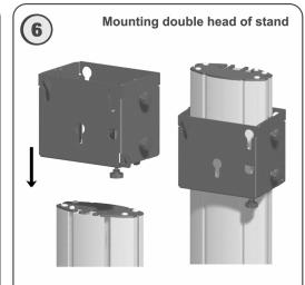
Slide the double head of the stand from the top downwards by using the T-ducts on both sides of the column. Tight the knobs on the right and left-hand side of the head to fix on a specific height.
