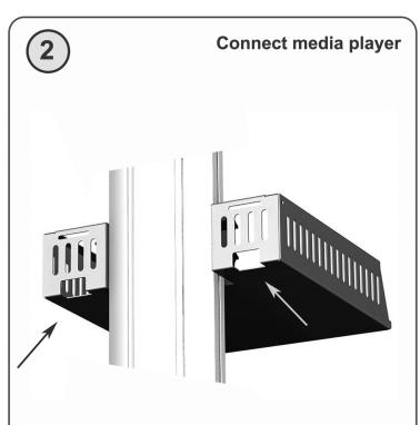
Place the media player as far as possible to the front of the media housing, this makes sure the air cooling can function optimally. Use the two slits at the back (see picture) to run the cables through.
