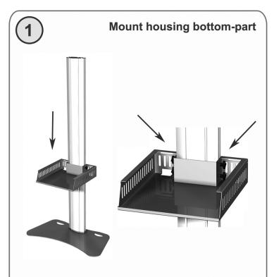
After a mounting bar is placed in both T-ducts on the sides, one can shove the bottom-part of the media housing over the column. When the required height has been reached, tighten the 4 knobs to fix its position.
