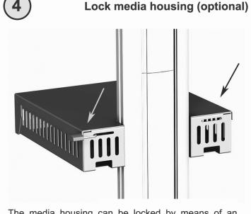
The media housing can be locked by means of an optional pad lock. This lock is run through the horizontal slit at the back, after which this lock is run though the sides of the bottom-, and top-part of the housing. One can choose whether to place a pad lock on the left and/or right side of the media housing.
