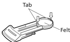
\* Wash the felt case with a neutral cleanser, and carefully wipe up any moisture before inserting it into the aroma base by following steps 1 and 2.
